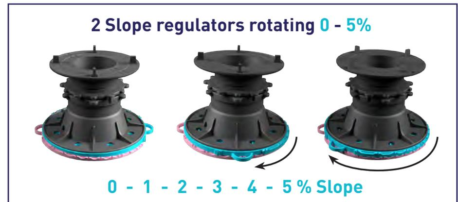
When several pieces are combined we can get all the inclination percentages lower than the maximum slope. We use several regulators to find the exact inclination. Each tab that we rotate to the regulator we add 0,25° of inclination.
